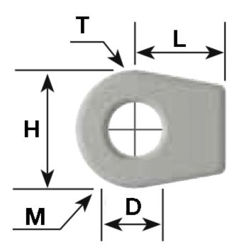
$\begin{array}{ll} D & = \varnothing 8,1 \\ H & = 17 \\ L & = 29 \\ M & = Metal \\ T (Thickness) = 10 \end{array}$
